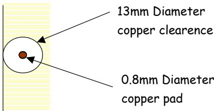
Target locations, 0.8mm (0.030") diameter pad in 13mm (0.50") diameter clearance of copper on top side of innerlayers
