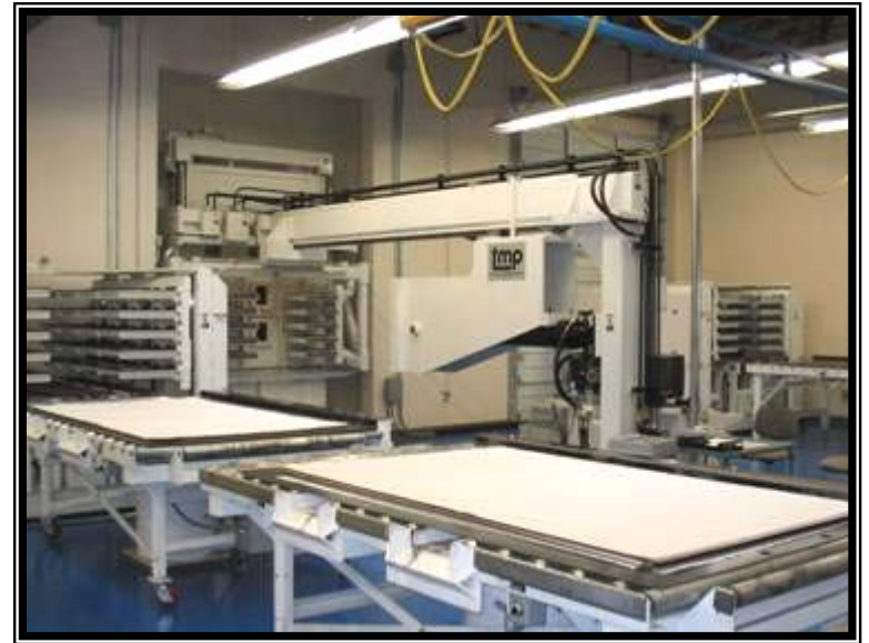
Neltec's large platen 50" x 80" PTFE press
