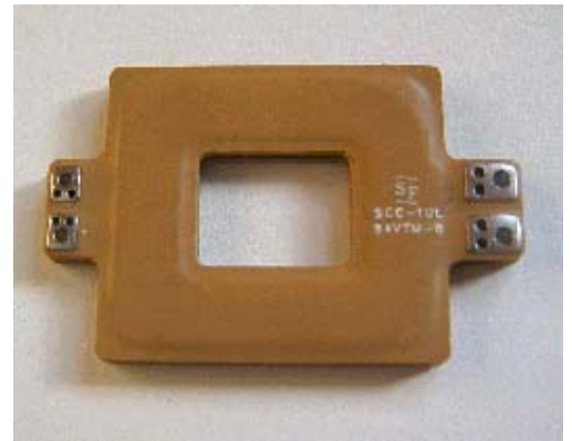
Planar transformer using heavy-metal flex circuitry
